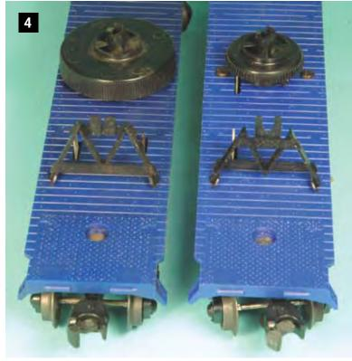
First, the winding spool was reduced from two inches to just over 1-3/8 inches in diameter and molded from a more durable plastic. This eliminated the problem with broken teeth.
