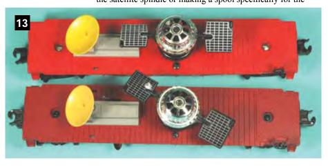
satellite with a smaller center hole. This would eliminate the wobble of the satellite as it rests on the spool.
