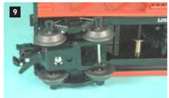
removed the shell. Once the shell was off, I removed the two outside pins that secure the levers. These pins are loose and without the shell in place can be easily pulled out.
