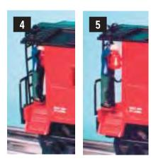
edge of the platform. The movement of the original version was quick and snappy as one would expect with a solenoid. On Lionel's new version, the man moves slowly back and forth. His movements are continuous as long as there is power to the track on which
