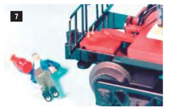
caboose. These pins carry current to the lantern held by the figure. The lantern is illuminated with an grain of wheat lamp. These last indefinitely and will most likely never need replacement. The lamp and its connections are molded within the figure. Should the lamp ever need replacement, the entire figure must be replaced.
