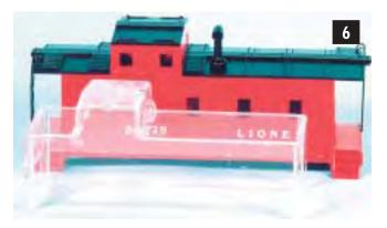
**Photo 6** shows the body with the ladders after having been removed from the frame. An interior clear shell is also shown. This piece is easily removed from the body after it is off the frame. **Photo 7** is a close-up of the figure. You can see the two small pins onto which it mounts at the rear of the
