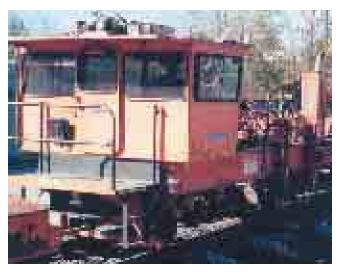
7. Next, a Tie-Remover-Inserter (TRI) removed the old ties from under the rails.
