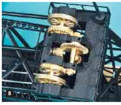
What I like so much about this system, is that you can at any time, simply lift the bridge with your hand and the weighs will slide down and hold it wherever you leave it. If the bridge were lifted by winding a thread or cable on a drum, this would not be possible.
