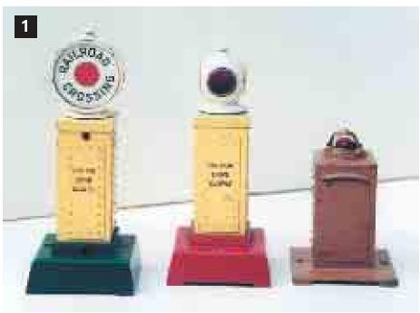
and shines through the celluloid. As the current flows, the nichrome wire heats up, causing the bimetallic arm to bend, and the switch opens. The lamp goes out, the wire cools, the switch closes, etc. The effect is a blinking light. It takes about 12 volts to operate, and the rate of the blinking depends upon the current as does the life of the bulb!
