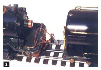
Now look at **photo 2** for the simple secret. The simple answer was to make a small loop out of a piece of scrap wire and run it through the brass trim on the pilot of the rear 260. Next, I hooked it over the rear tender coupler of the lead unit.
