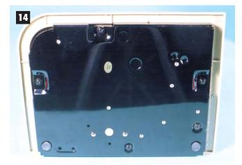
**Photo 14** shows the bottom of the latest version. Here you can see the five screws which hold the tan plastic in place. There is also the obligatory Made in China sticker. The base also has two rubber feet at the back edge and a third one centered towards the front.
