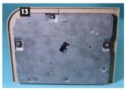
to the metal base plate. These must certainly torment a service station attempting to make repairs. I much prefer screws or machine nuts to speed nuts. Speed nuts show no concern for whoever might have to make a repair.
