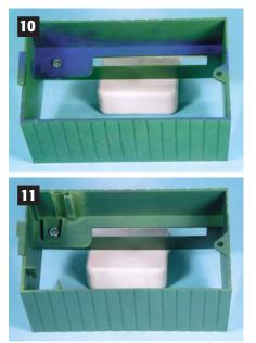
molded in green plastic and painted. Notice in the upper left hand corner of the photo, the track that is molded into the front to accept the plastic lamp holder. Notice also the two hooks molded into the rear corner to guide the wires. One other difference with the new one is the tab on the side. The tab now has a step in it and I have no idea why this change was made.
