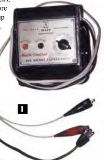
easy to reverse the polarity (i.e., reverse the hot and ground leads) to the track/loco to test bell and whistle activation on some of the newer equipment.
