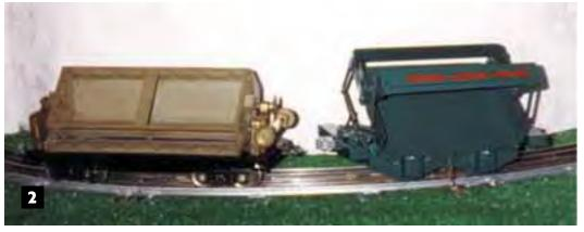
The mechanism of the original Lionel 2-1/8-inch dump car (left) is a worm gear with two knobs on one end, while the Buddy "L" construction car uses levers to dump its load.
