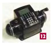
interesting additions. First, the YardBoss has the functions of two CAB-1 controllers built into it. This means that you can address two separate engines at the same time without readdressing. **Photo 12**
