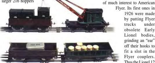
Flyer. Its first ones in 1926 were made by putting Flyer trucks under obsolete Early Lionel bodies, grinding an "ear" off their hooks to fit a slot in the Flyer couplers. Thus the Lionel 12 gondola became a Flyer 4017 sand
