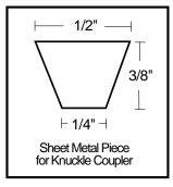
could drill into the coupler head and attach the bar to it with a #2 sheet metal screw). Make another hole on the other end where indicated in the diagram, just big enough to thread the #4-40 1/4-inch machine screw securely into it. Fashion the little sheet metal plate that will go over the coupler opening (see diagram).
