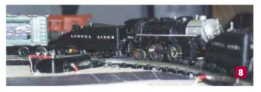
my tenders are spruced up with die-cast trucks, porthole lenses to fit on the backup lights, and handrails fashioned from some extra handrail wire — similar to those on the scale slope-back tenders.
